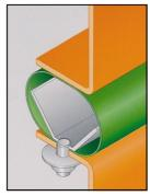
The illustrations on the left depict the patented sealing system **NICROFLEX - HIPERFORM** in uncompressed and compressed condition. In uncompressed condition ( damper open ) the internal, vee – shaped, lateral stabiliser makes contact with and supports the seals metal loop thus preventing gas flow induced vibrations. In compressed condition (damper closed )the metal loops flatten and bulge outwards, thereby enhancing their ability to withstand high pressure differentials.
