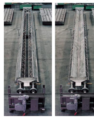
The operating temperature may rise up to 700 degrees C. However, since all the members of the lattice support structure are evenly swept by the hot flue gases they heat up uniformly and thereby any distortions are averted.
