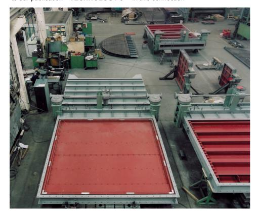
The picture shows three ,out of a total of six, guillotines supplied in this case, during final assembly and testing at the Rauenstein
