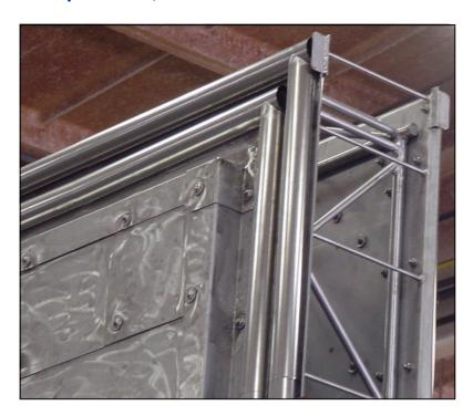
The lattice structure reinforced blade with cardanically attached, free floating cover plates remains free of distortions when exposed to high and rapidly changing temperatures. High temperature gas flows continuously through the blade's latticed support structure, all parts of which heat up uniformly.
