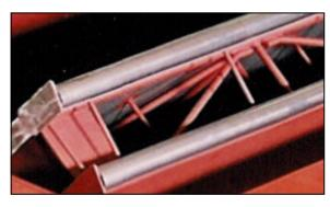
The lattice structure reinforced blade with cardanically attached, free floating cover plates remains free of distortions when exposed to high and rapidly changing temperatures. High temperature gas flows continuously through the blade's latticed support structure, all parts of which heat up uniformly.
