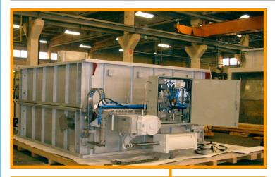
The picture above depicts one of the **RAUMAG - JANICH** supplied dampers during trial runs at the Rauenstein works. They will be used for flow modulation and rerouting operations of the turbine exhaust gas. With seal air, a gastight, man safe shut – off can be achieved.
