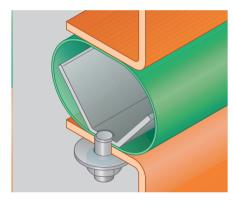
The drawing depicts a cross section through the diverter. At its outlet it is equipped with a blanking plate, which is positioned outside the duct during normal operation. The pivoting blade carries a double seal on each side with which it makes contact with the respective landing bars in the end positions. With seal air, 100% tightness is achieved.
