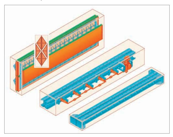
The lattice supported blade design DBP in conjunction with the highly resilient, new sealing system NICROFLEX-HIPERFORM DBPa, facilitate long span damper blades. It is therefore possible to design louver- and tandem dampers without intermediate bearing supports in the duct. Such dampers are simpler in design as conventional dampers and also less prone to operational trouble.
