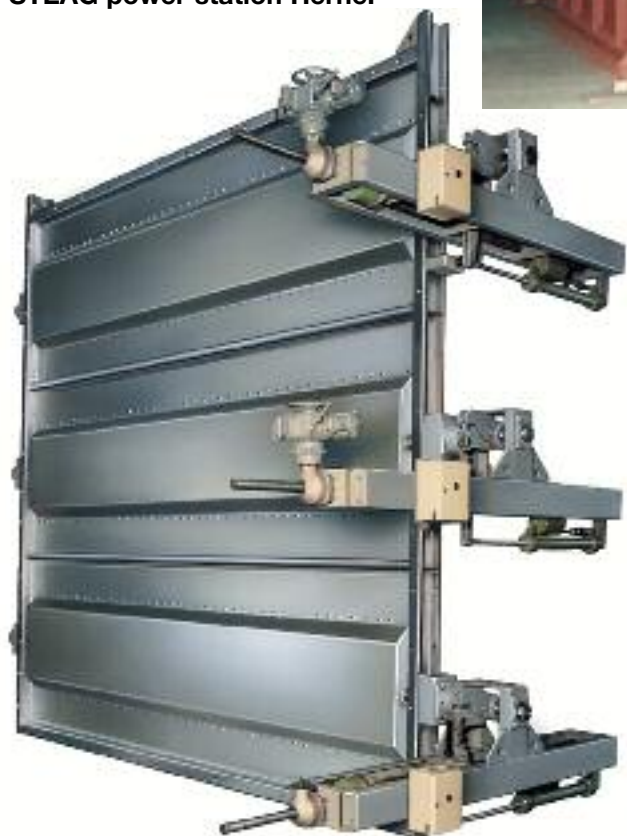
Illustration top, right: Louvre damper DN 5600 mm with NICROFLEX sealing system. Rating: t = 400\text{ }^{\circ}\text{C} , p\text{ diff. } 90\text{ mbar} Material: 15 Mo 3. Supplied for the DeNOx plant in the STEAG power station Herne.
