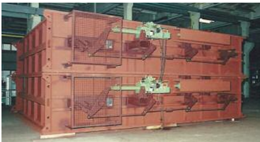
Illustration above: Two louvre dampers NS 6200 x 6200 mm undergoing leak-tightness testing at the Rauenstein works. Supplied for the flue gas desulphurising plant at the Boxberg power station. The dampers are operated by a hydraulic drive with an emergency operation feature.
