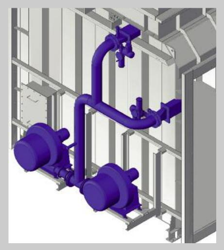
In conjunction with a double seal, a 100% shut-off of the hot gas flow is achieved by the introduction of purge air between the two sealing planes when the damper blade is closed. In the process, the purge air pressure must be greater than the pressure of the gas being shut off.
