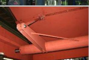
Illustration above: **Flap damper NS 7480 x 5300 mm.** Supplied for the **De-NOx plant at the AMER power station in Holland.** The lattice supported blade is driven via a toggle system (insert). 100% gas-tight using the NICROFLEX-HIPERFORM sealing system.
